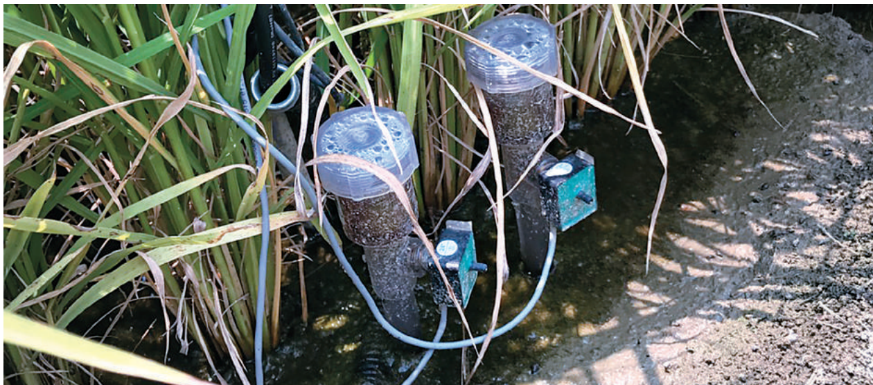
▲ 土壤水分含量感測器能有效控制灌溉自動閘門，以花最少的人力，放最少的水，去灌溉最多的面積。Soil moisture sensor allows automated irrigation control, which maximizes irrigation area for the given volume of water while requiring little to no labor.
